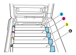
**3.** Pull the colored toner release lever on the cartridge to be replaced towards the front of the printer.
