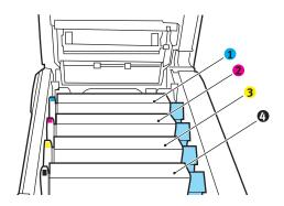
**3.** Lift the image drum, complete with its toner cartridge, out of the printer. Discard it in accordance with your local regulations.
