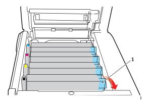
**4.** Lift the right-hand end of the cartridge. Then, pull the cartridge to the right to release the left-hand end. Remove the toner cartridge. Discard it in accordance with your local regulations.
