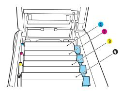
**3.** Lift each of the image drum units out of the printer. Place them on a *flat* surface in a safe place away from direct sources of heat and light.
