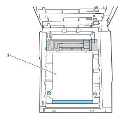
**CAUTION!** Do not use any sharp or abrasive objects to separate sheets from the belt. This may damage the belt surface.
