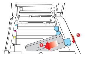
**8.** Lower the right end of the cartridge into the image drum unit. Press it firmly down in place. Then, push the colored lock lever back to open the toner slot and lock it in place.
