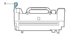
**8.** Push the blue retaining lever (2) toward the rear of the printer to lock the fuser in place.
